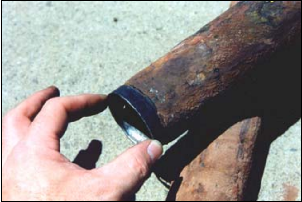
Photo “H” Note black iron oxide on portion of stub end.
